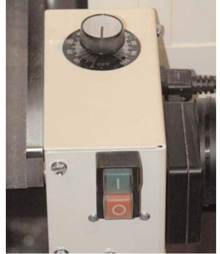
Photo.7: The controls consist of on and off switches and a variable speed control for the conveyor belt
