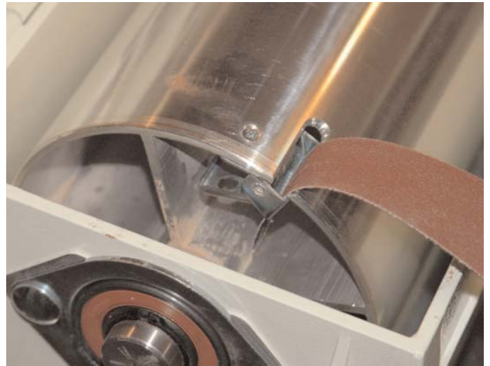
Photo.4: The clip on the out-board end of the drum is easy to access
