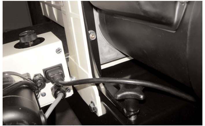
Photo.3: Bolt at bottom centre is one of four that secures the vertical drum support frame. The drum alignment knob as is at bottom right under the motor.
