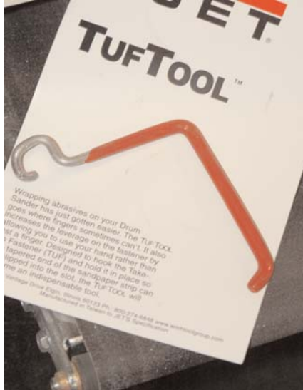
Photo.6: The TUF tool makes it easier to attach the inboard end of the strip
