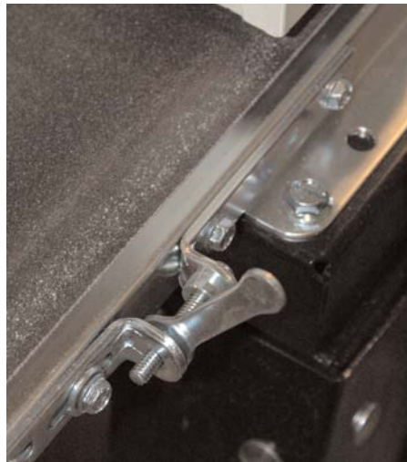
Photo.8: Captive spanners are provided for adjustment of conveyor belt tracking
