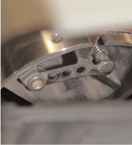
Photo.5: The clip on the inboard end of the drum (seen here through a void in the frame) is a little harder to reach but a special tool is provided to help.
