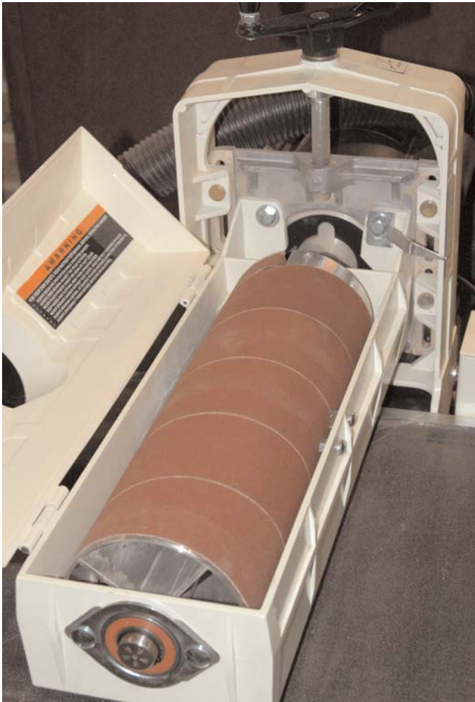
Photo.2: Swinging the dust cover back reveals the drum and sanding strip. The frame at the back carries the main bearing and height adjustment mechanism and is pivoted to allow the outboard end of the drum (nearest camera) to be raised or lowered
