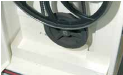
Photo.7&8: There are two swarf trays — back of the table and inside the base
