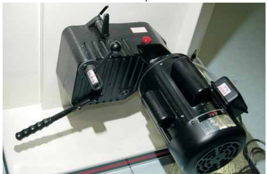
Photo.6: The motor drives the machine through a gearbox— the gear knob is in the centre, the motor lifting lever is on the left and the securing knob is at the top.
