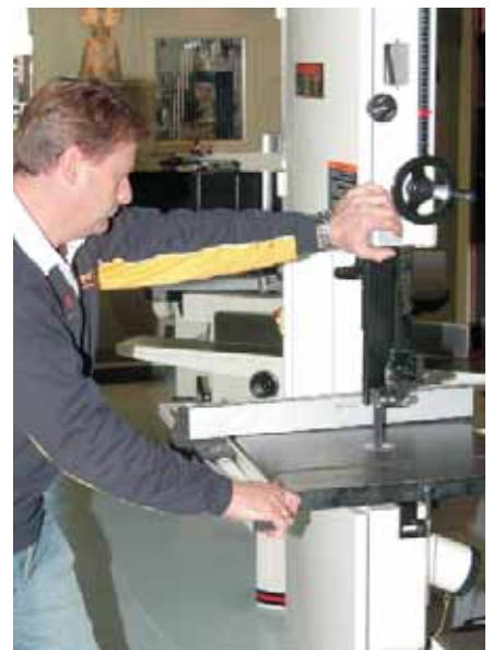
Photo.4: Jason Burgmann (Benchworks, Emu Plains, NSW) does the shove test
