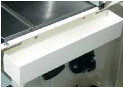
Photo.7&8: There are two swarf trays — back of the table and inside the base
