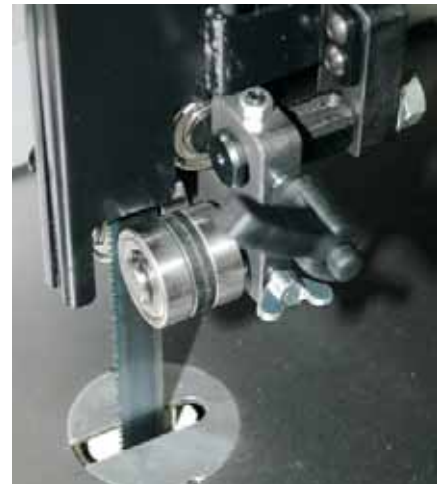
Photo.10: Machine uses quickly adjusted US Carter guides
