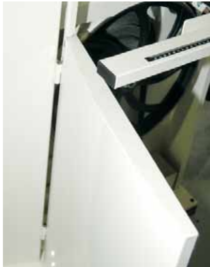
Photo.5: New curved doors should reduce chances of vibration
