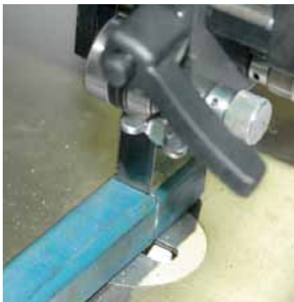
Photo.9: Cutting is fast and accurate — note fine tooth 'metal' blade
