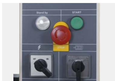
2 blade speeds via 2-step motor
