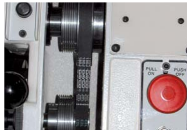
Two belt stages for high torque when turning large diameter workpieces
