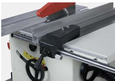
Rigid rip fence with round bar guide and integrated micro-adjustment
