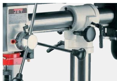
Rack and pinion fine adjustment of swing
