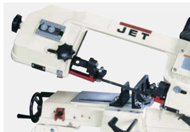
Fully adjustable ball bearing blade guides
