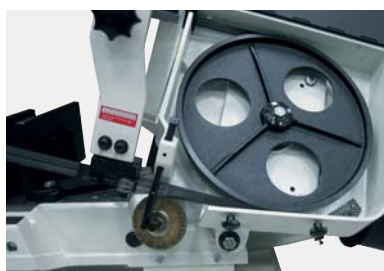
Brass brush wheel for saw blade cleaning
