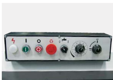
Central control unit
