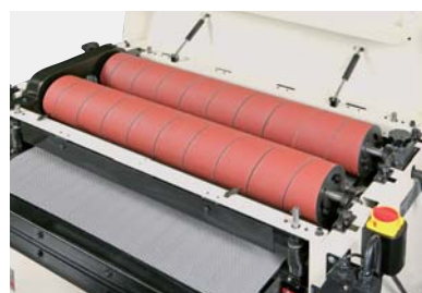
2 sanding drums for roughing and finishing in one operation
