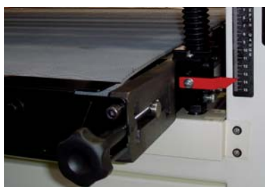
The conveyor bed is guided on 4 solid jackscrews
