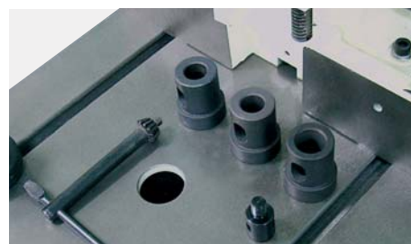
Chisel shank adapters 5/8", 3/4", 13/16", long chuck key and spindle extension
